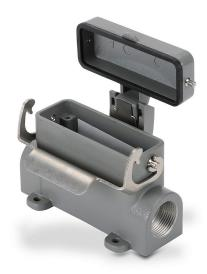
ZIPport surface mount housing, single lever, standard, connector housing size 16A, (2) Pg 16 threaded holes, heavy-duty die cast aluminum. For use with ZIPport size 16A 2-peg connector housings.
