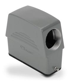
ZIPport hood housing, 2-peg, side entry, connector housing size 16A, (1) Pg 21 threaded hole, high construction, heavy-duty die cast aluminum. For use with ZIPport size 16A single lever connector housings.
