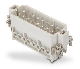
ZIPport male insert, connector housing size 16A, 16-pole, screw terminals, accepts wire size 20-14 AWG, 16 amp, 600 VAC/VDC, poles numbered 1 to 16. For use with ZIPport multi-wire housings.
