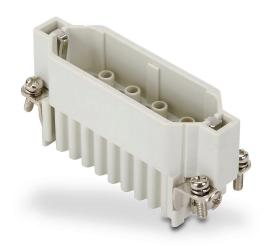
ZIPport male insert, connector housing size 16A, 25-pole, crimped contact, 10 amp, 600 VAC/VDC, poles numbered 1 to 25. For use with ZIPport multi-wire housings. Requires 10 amp male contacts ZP-MC-CC-M10A-xxx.
