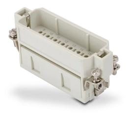
ZIPport male insert, connector housing size 16A, 16-pole, crimped contact, 16 amp, 600 VAC/VDC, poles numbered 1 to 16. For use with ZIPport multi-wire housings. Requires 16 amp male contacts ZP-MC-CC-M16A-xxx.
