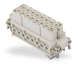
ZIPport female insert, connector housing size 16A, 16-pole, screw terminals, accepts wire size 20-14 AWG, 16 amp, 600 VAC/VDC, poles numbered 1 to 16. For use with ZIPport multi-wire housings.
