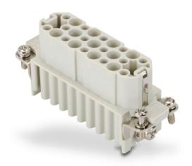
ZIPport female insert, connector housing size 16A, 25-pole, crimped contact, 10 amp, 600 VAC/VDC, poles numbered 1 to 25. For use with ZIPport multi-wire housings. Requires 10 amp female contacts ZP-MC-CC-F10A-xxx.
