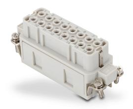
ZIPport female insert, connector housing size 16A, 16-pole, crimped contact, 16 amp, 600 VAC/VDC, poles numbered 1 to 16. For use with ZIPport multi-wire housings. Requires 16 amp female contacts ZP-MC-CC-F16A-xxx.
