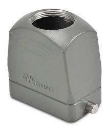
ZIPport hood housing, 2-peg, top entry, connector housing size 10B, (1) Pg 29 threaded hole, high construction, heavy-duty die cast aluminum. For use with ZIPport size 10B single lever connector housings.
