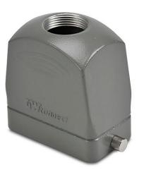
ZIPport hood housing, 2-peg, top entry, connector housing size 10B, (1) Pg 21 threaded hole, high construction, heavy-duty die cast aluminum. For use with ZIPport size 10B single lever connector housings.
