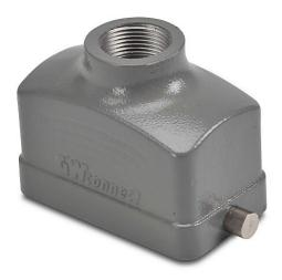
ZIPport hood housing, 2-peg, top entry, connector housing size 10B, (1) Pg 16 threaded hole, heavy-duty die cast aluminum. For use with ZIPport size 10B single lever connector housings.
