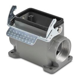
ZIPport surface mount housing, single lever, connector housing size 10B, (2) Pg 29 threaded holes, high construction, heavy-duty die cast aluminum. For use with ZIPport size 10B 2-peg connector housings.
