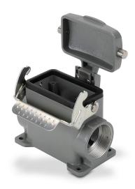
ZIPport surface mount housing, single lever, standard, connector housing size 10B, (2) Pg 29 threaded holes, high construction, heavy-duty die cast aluminum. For use with ZIPport size 10B 2-peg connector housings.
