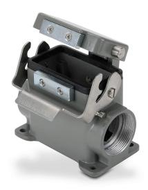
ZIPport surface mount housing, single lever, automatic closing, connector housing size 10B, (2) Pg 29 threaded holes, heavy-duty die cast aluminum. For use with ZIPport size 10B 2-peg connector housings.
