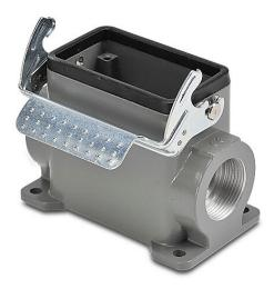
ZIPport surface mount housing, single lever, connector housing size 10B, (2) Pg 21 threaded holes, high construction, heavy-duty die cast aluminum. For use with ZIPport size 10B 2-peg connector housings.
