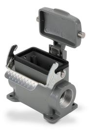
ZIPport surface mount housing, single lever, standard, connector housing size 10B, (2) Pg 21 threaded holes, high construction, heavy-duty die cast aluminum. For use with ZIPport size 10B 2-peg connector housings.
