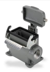
ZIPport surface mount housing, single lever, standard, connector housing size 10B, (2) Pg 21 threaded holes, high construction, heavy-duty die cast aluminum. For use with ZIPport size 10B 2-peg connector housings.
