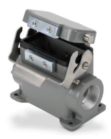
ZIPport surface mount housing, single lever, automatic closing, connector housing size 10B, (2) Pg 21 threaded holes, heavy-duty die cast aluminum. For use with ZIPport size 10B 2-peg connector housings.
