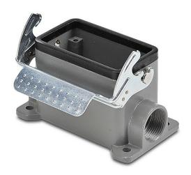
ZIPport surface mount housing, single lever, connector housing size 10B, (2) Pg 16 threaded holes, heavy-duty die cast aluminum. For use with ZIPport size 10B 2-peg connector housings.
