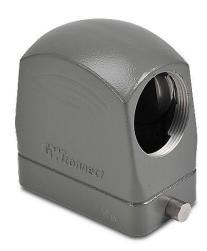
ZIPport hood housing, 2-peg, side entry, connector housing size 10B, (1) Pg 29 threaded hole, high construction, heavy-duty die cast aluminum. For use with ZIPport size 10B single lever connector housings.
