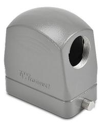
ZIPport hood housing, 2-peg, side entry, connector housing size 10B, (1) Pg 21 threaded hole, high construction, heavy-duty die cast aluminum. For use with ZIPport size 10B single lever connector housings.
