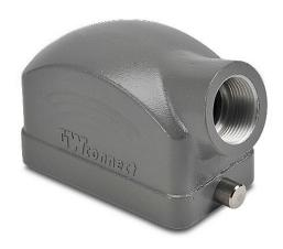
ZIPport hood housing, 2-peg, side entry, connector housing size 10B, (1) Pg 16 threaded hole, heavy-duty die cast aluminum. For use with ZIPport size 10B single lever connector housings.
