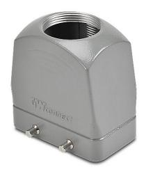
ZIPport hood housing, 4-peg, top entry, connector housing size 10B, (1) Pg 29 threaded hole, high construction, heavy-duty die cast aluminum. For use with ZIPport size 10B double lever connector housings.
