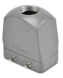
ZIPport hood housing, 4-peg, top entry, connector housing size 10B, (1) Pg 21 threaded hole, high construction, heavy-duty die cast aluminum. For use with ZIPport size 10B double lever connector housings.
