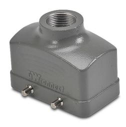
ZIPport hood housing, 4-peg, top entry, connector housing size 10B, (1) Pg 16 threaded hole, heavy-duty die cast aluminum. For use with ZIPport size 10B double lever connector housings.
