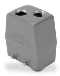
ZIPport hood housing, 4-peg, top entry, connector housing size 10B, (2) Pg 13.5 threaded hole, high construction, heavy-duty die cast aluminum. For use with ZIPport size 10B double lever connector housings.
