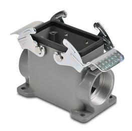
ZIPport surface mount housing, double lever, connector housing size 10B, (2) Pg 29 threaded holes, high construction, heavy-duty die cast aluminum. For use with ZIPport size 10B 4-peg connector housings.
