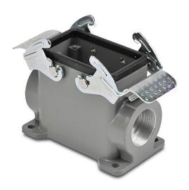
ZIPport surface mount housing, double lever, connector housing size 10B, (2) Pg 21 threaded holes, high construction, heavy-duty die cast aluminum. For use with ZIPport size 10B 4-peg connector housings.
