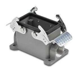
ZIPport surface mount housing, double lever, connector housing size 10B, (2) Pg 16 threaded holes, heavy-duty die cast aluminum. For use with ZIPport size 10B 4-peg connector housings.
