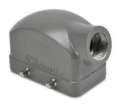
ZIPport hood housing, 4-peg, side entry, connector housing size 10B, (1) Pg 16 threaded hole, heavy-duty die cast aluminum. For use with ZIPport size 10B double lever connector housings.
