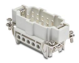
ZIPport male insert, connector housing size 10B, 10-pole, screw terminals, accepts wire size 20-12 AWG, 16 amp, 600 VAC/VDC, poles numbered 1 to 10. For use with ZIPport multi-wire housings.
