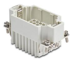
ZIPport male insert, connector housing size 10B, 42-pole, crimped contact, 10 amp, 600 VAC/VDC, poles numbered 1 to 42. For use with ZIPport multi-wire housings. Requires 10 amp male contacts ZP-MC-CC-M10A-xxx.
