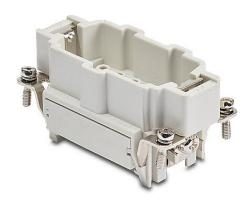
ZIPport male insert, connector housing size 10B, 10-pole, crimped contact, 16 amp, 600 VAC/VDC, poles numbered 1 to 10. For use with ZIPport multi-wire housings. Requires 16 amp male contacts ZP-MC-CC-M16A-xxx.
