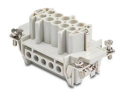
ZIPport female insert, connector housing size 10B, 10-pole, screw terminals, accepts wire size 20 - 12 AWG, 16 amp, 600 VAC/VDC, poles numbered 1 to 10. For use with ZIPport multi-wire housings.
