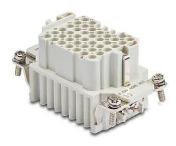
ZIPport female insert, connector housing size 10B, 42-pole, crimped contact, 10 amp, 600 VAC/VDC, poles numbered 1 to 42. For use with ZIPport multi-wire housings. Requires 10 amp female contacts ZP-MC-CC-F10A-xxx.
