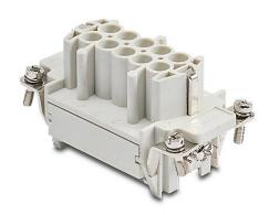
ZIPport female insert, connector housing size 10B, 10-pole, crimped contact, 16 amp, 600 VAC/VDC, poles numbered 1 to 10. For use with ZIPport multi-wire housings. Requires 16 amp female contacts ZP-MC-CC-F16A-xxx.
