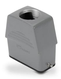
ZIPport hood housing, 2-peg, top entry, connector housing size 10A, (1) Pg 21 threaded hole, high construction, heavy-duty die cast aluminum. For use with ZIPport size 10A single lever connector housings.
