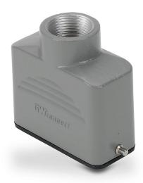
ZIPport hood housing, 2-peg, top entry, connector housing size 10A, (1) Pg 16 threaded hole, heavy-duty die cast aluminum. For use with ZIPport size 10A single lever connector housings.
