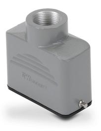
ZIPport hood housing, 2-peg, top entry, connector housing size 10A, (1) Pg 13.5 threaded hole, heavy-duty die cast aluminum. For use with ZIPport size 10A single lever connector housings.
