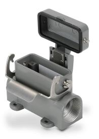
ZIPport surface mount housing, single lever, standard, connector housing size 10A, (2) Pg 21 threaded holes, heavy-duty die cast aluminum. For use with ZIPport size 10A 2-peg connector housings.
