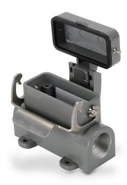
ZIPport surface mount housing, single lever, standard, connector housing size 10A, (2) Pg 16 threaded holes, heavy-duty die cast aluminum. For use with ZIPport size 10A 2-peg connector housings.
