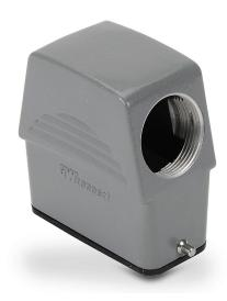
ZIPport hood housing, 2-peg, side entry, connector housing size 10A, (1) Pg 21 threaded hole, high construction, heavy-duty die cast aluminum. For use with ZIPport size 10A single lever connector housings.
