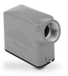
ZIPport hood housing, 2-peg, side entry, connector housing size 10A, (1) Pg 16 threaded hole, heavy-duty die cast aluminum. For use with ZIPport size 10A single lever connector housings.
