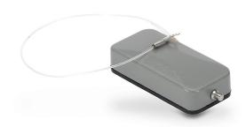
ZIPport cover housing, 2-peg, connector housing size 10A, heavy-duty die cast aluminum. For use with ZIPport size 10A single lever connector housings.
