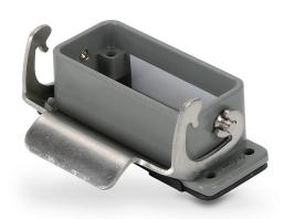
ZIPport bulkhead housing, single lever, connector housing size 10A, heavy-duty die cast aluminum. For use with ZIPport size 10A 2-peg connector housings.
