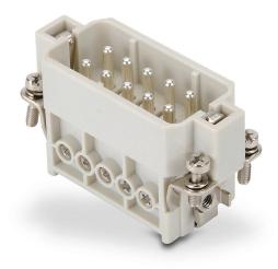
ZIPport male insert, connector housing size 10A, 10-pole, screw terminals, accepts wire size 20-14 AWG, 16 amp, 600 VAC/VDC, poles numbered 1 to 10. For use with ZIPport multi-wire housings.
