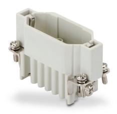
ZIPport male insert, connector housing size 10A, 15-pole, crimped contact, 10 amp, 600 VAC/VDC, poles numbered 1 to 15. For use with ZIPport multi-wire housings. Requires 10 amp male contacts ZP-MC-CC-M10A-xxx.
