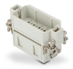
ZIPport male insert, connector housing size 10A, 10-pole, crimped contact, 16 amp, 600 VAC/VDC, poles numbered 1 to 10. For use with ZIPport multi-wire housings. Requires 16 amp male contacts ZP-MC-CC-M16A-xxx.
