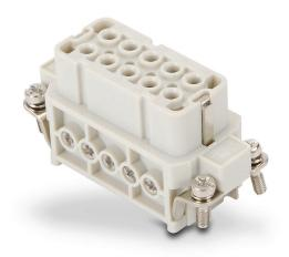
ZIPport female insert, connector housing size 10A, 10-pole, screw terminals, accepts wire size 20-14 AWG, 16 amp, 600 VAC/VDC, poles numbered 1 to 10. For use with ZIPport multi-wire housings.
