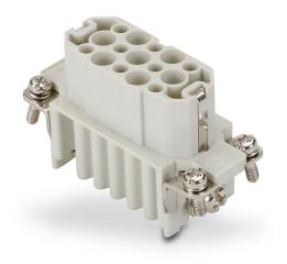
ZIPport female insert, connector housing size 10A, 15-pole, crimped contact, 10 amp, 600 VAC/VDC, poles numbered 1 to 15. For use with ZIPport multi-wire housings. Requires 10 amp female contacts ZP-MC-CC-F10A-xxx.
