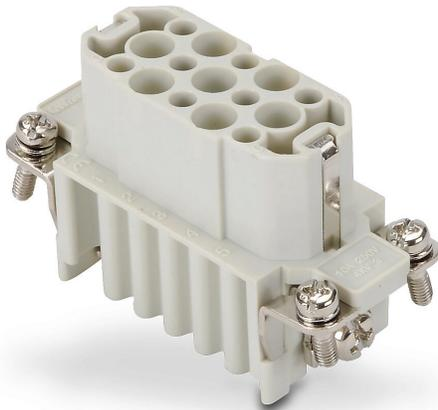
ZIPport female insert, connector housing size 10A, 15-pole, crimped contact, 10 amp, 600 VAC/VDC, poles numbered 1 to 15. For use with ZIPport multi-wire housings. Requires 10 amp female contacts ZP-MC-CC-F10A-xxx.
