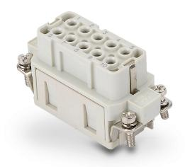
ZIPport female insert, connector housing size 10A, 10-pole, crimped contact, 16 amp, 600 VAC/VDC, poles numbered 1 to 10. For use with ZIPport multi-wire housings. Requires 16 amp female contacts ZP-MC-CC-F16A-xxx.
